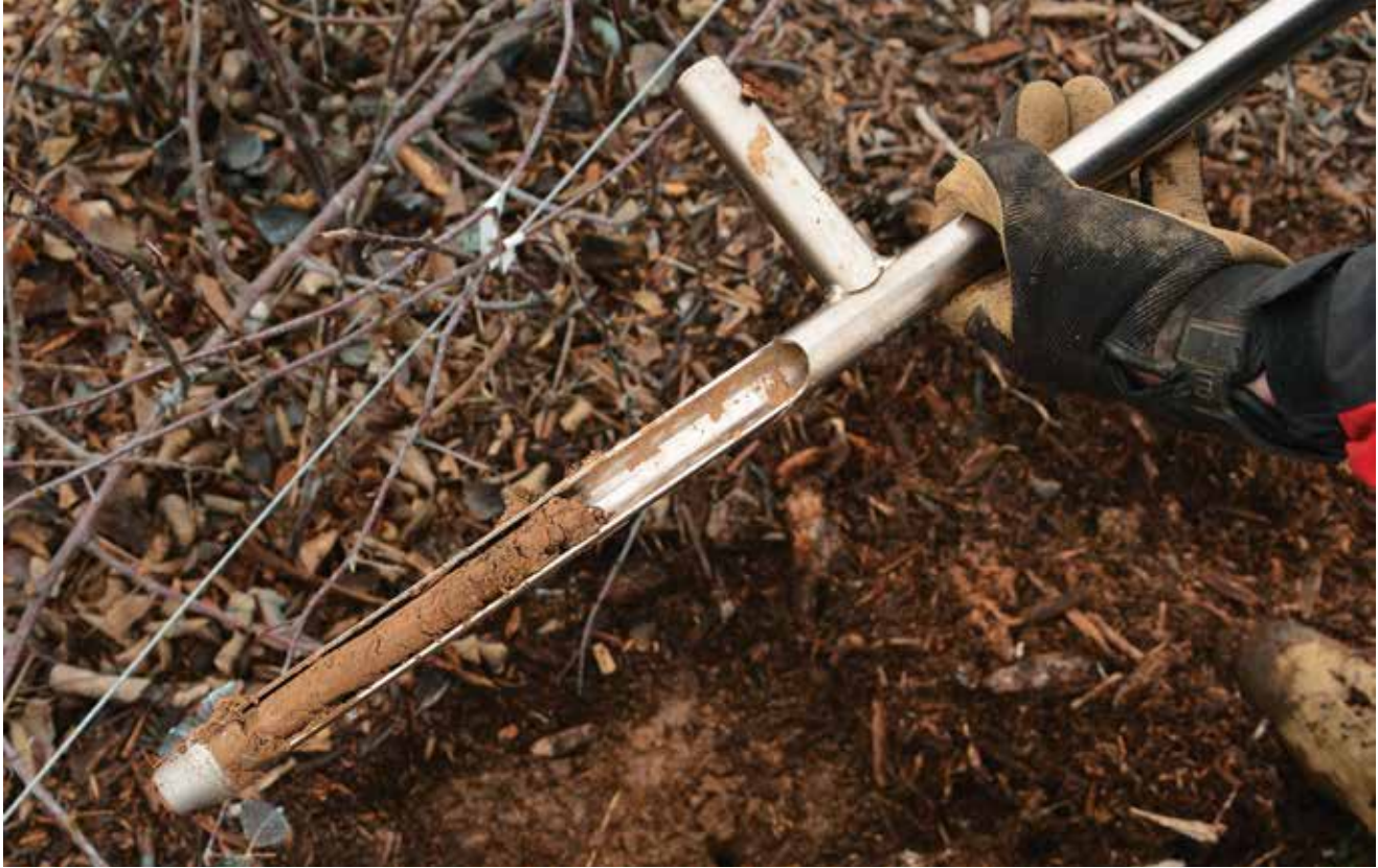
A soil probe used to collect multiple six-inch soil cores, which are mixed together to generate a sample. Photo by Luke Freeman.
